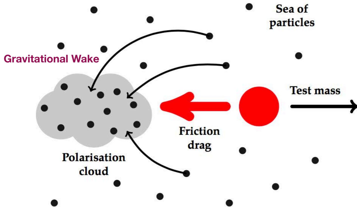
$$[\delta\psi]_{\text{dressed}} = \frac{[\delta\psi]_{\text{bare}}}{|\epsilon(\omega)|}$$
